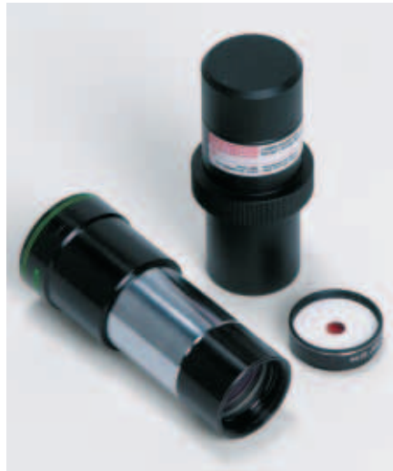
Above, left: The Barlowed laser consists of three main pieces: an ordinary laser collimator, a Barlow lens, and a screen consisting of a cardboard disk mounted in a color planet filter (red, in this case).
