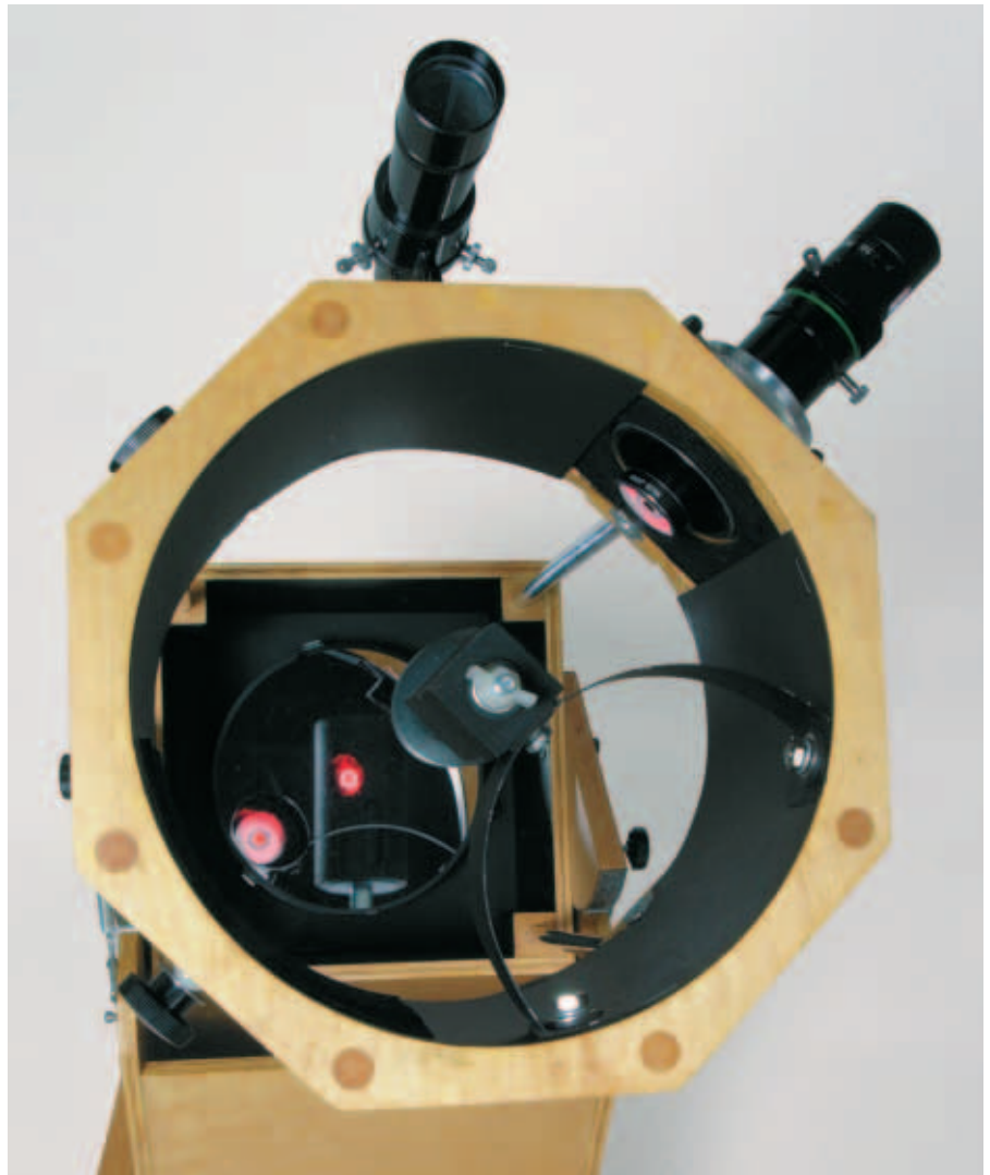
A standard laser collimator can yield unsatisfactory optical alignment. However, using such a device with an ordinary Barlow lens allows collimation on a par with the precision obtained with a good Cheshire eyepiece. All photographs are by Craig Michael Utter, Sky & Telescope .
