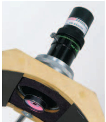
Above, left: The Barlowed laser consists of three main pieces: an ordinary laser collimator, a Barlow lens, and a screen consisting of a cardboard disk mounted in a color planet filter (red, in this case).
